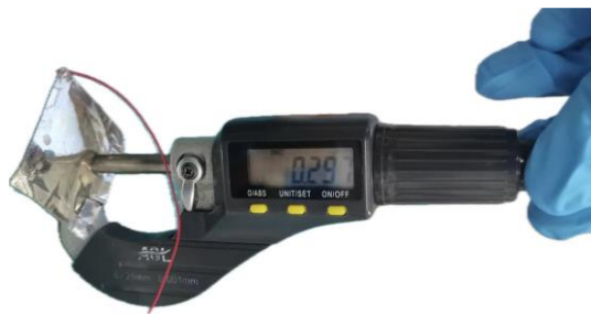
Figure 3.3 Optical photo showing the thickness of the sensor.
